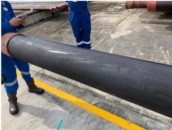
RC-12 after 29 days exposed to the elements. No visible signs of corrosion. Hard cured and NON-GREASY surface.
