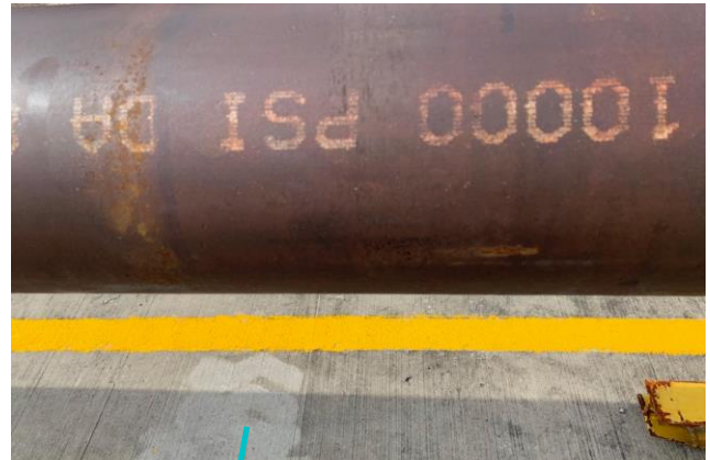
Synergen 501 TR after 29 days exposed to the elements. Remained greasy with minor rust breakout observed
